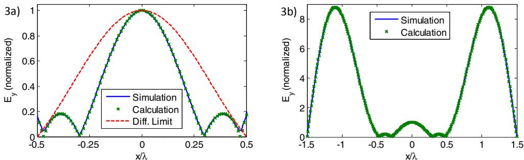
Figure 3. 2 plots comparing simulated and calculated profiles for  $E_y(x)$ . a) A close up showing the subwavelength peak, compared alongside the diffraction-limited sinc function. b) A comparison of the field profile across the waveguide.
