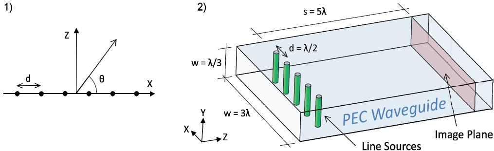
Figure 1. A diagram showing a generic antenna array (elements denoted by black dots).
